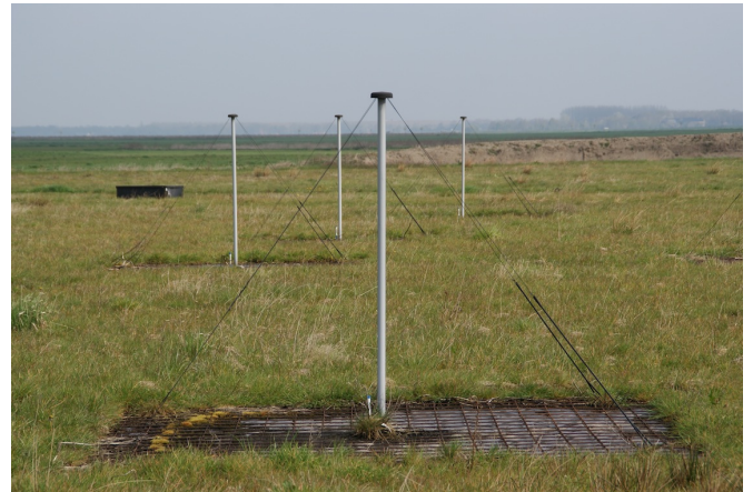
Fig. 2. Low-band antennas at the central core of LOFAR, the Superterp. In the background the black box of a LORA particle detector can be seen.
