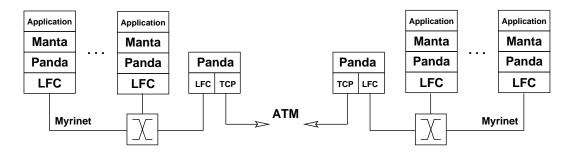
Figure 2: Wide area communication based on Panda
