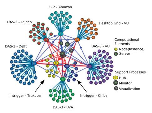
Figure 9. Communication structure of the worldwide divide-and-conquer experiment. Nodes in this graph represent processes, edges represent connections. The experiment contains both nodes performing the computation, as well as a number of support processes which allow communication to pass through firewalls, monitor the communication, and produce this image. Each color represents a different location.
