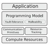
Figure 1. Abstract system hierarchy with resource tracking and communication primitives being the central low-level primitives for developing fault-tolerant and malleable programming models and applications.
