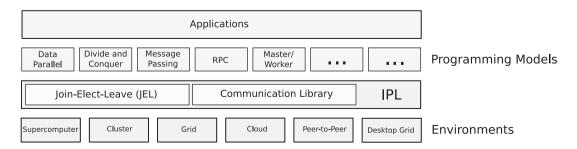
Figure 3. Position of JEL in the Ibis grid programming software stack.
