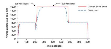
Figure 8. Join/fail test run on four clusters across the DAS-3 grid. Half of the nodes only start after 200 s, and crash after 400 s.
