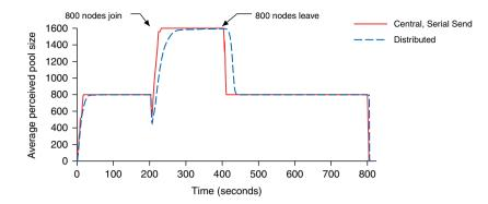
Figure 7. Join/leave test run on four clusters across the DAS-3 grid. Half of the nodes only start after 200 s, and leave after 400 s.
