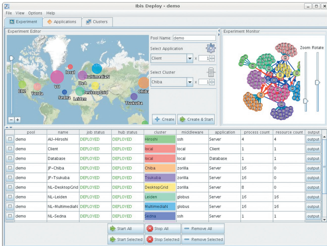
Figure 3. The IbisDeploy GUI lets users load applications and resources (top middle) and keep track of running processes (bottom half). The top left of the figure shows the locations of available resources; the top right shows the SmartSockets network consisting of hubs and compute nodes. A video presentation is available at www.cs.vu.nl/ibis/demos.html .
